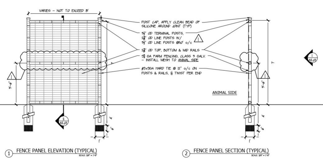
NOTE: MESH AND HARDWARE TO BE GALVANIZED AND BLACK VINYL COATED POSTS AND RAILS TO BE GALVANIZED AND PAINTED BLACK
